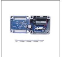
4. Open the front panel of the controller and take out the battery holder. Install 4\*AA batteries in the battery holder and plug it back in.
