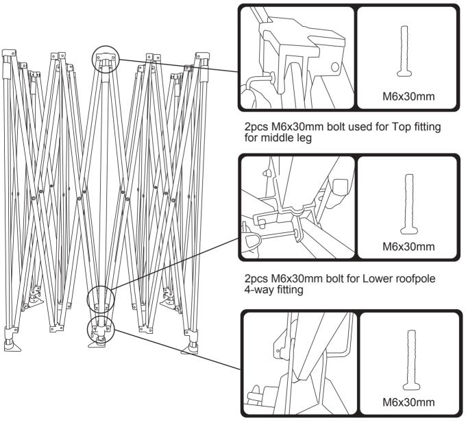
2pcs M6x30mm bolt used for fitting for middle leg
