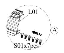
Pre-sliding bolt S01 x 7 before assembling L01, they will be used for assemble L10L, L10R, W16B,L13A in following steps.
