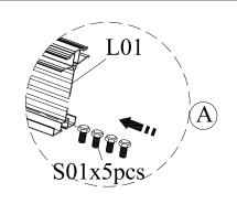
Pre-sliding bolt S01 x 5 before assembling L01, they will be used for assemble L10L, L10R, L13A in following steps.
